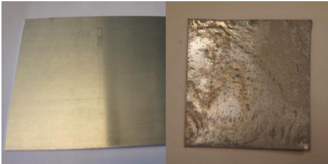
Figure 2 The zinc sheet prior to the leaching (left) and after the leaching (right).
